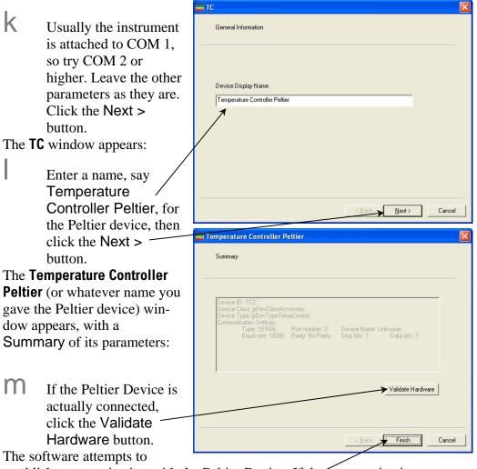
establish communication with the Peltier Device. If the communication attempt fails, an error message appears. Verify that the correct COM port is used and that all cables are firmly attached.
