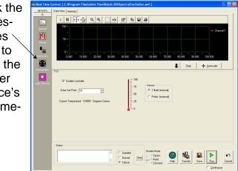
4 Modify the Peltier devices parameters as desired, while viewing the real-time data.
