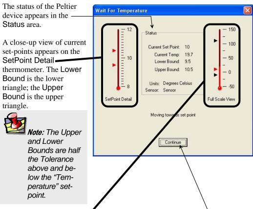
A full-range thermometer appears in the Full Scale View. Maximum and minimum possible set-points are black triangles.
