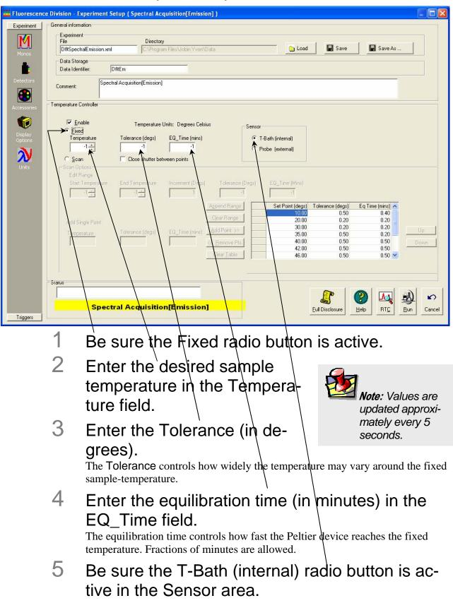
The Peltier device does not use the Probe (external) sensor.
