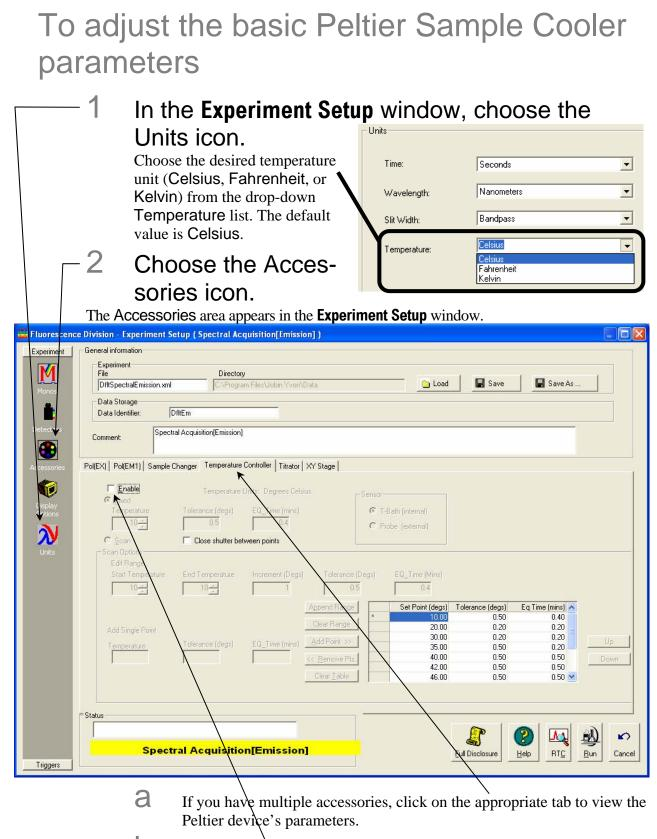
**D** Check the Enable checkbox to activate the Peltier device. Some of the parameters become active, as shown below:
